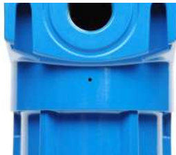
Pressure relief hole gives an audible warning if any attempt is made to remove filter bowl whilst under pressure.
